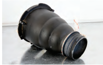
An example of a homemade snoot using just a plastic water bottle and a device designed to measure spaghetti servings for the aperture control.
