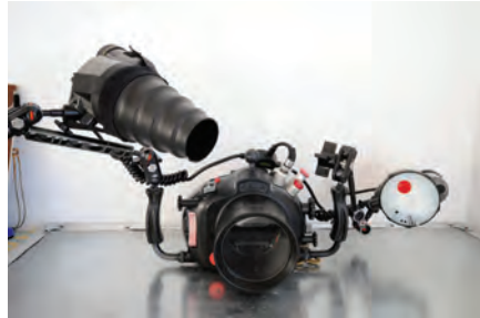
A wide angle set-up uses a wider snoot for more coverage.
