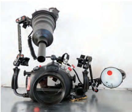
Set-up for macro photography with a narrow snoot fixture.
